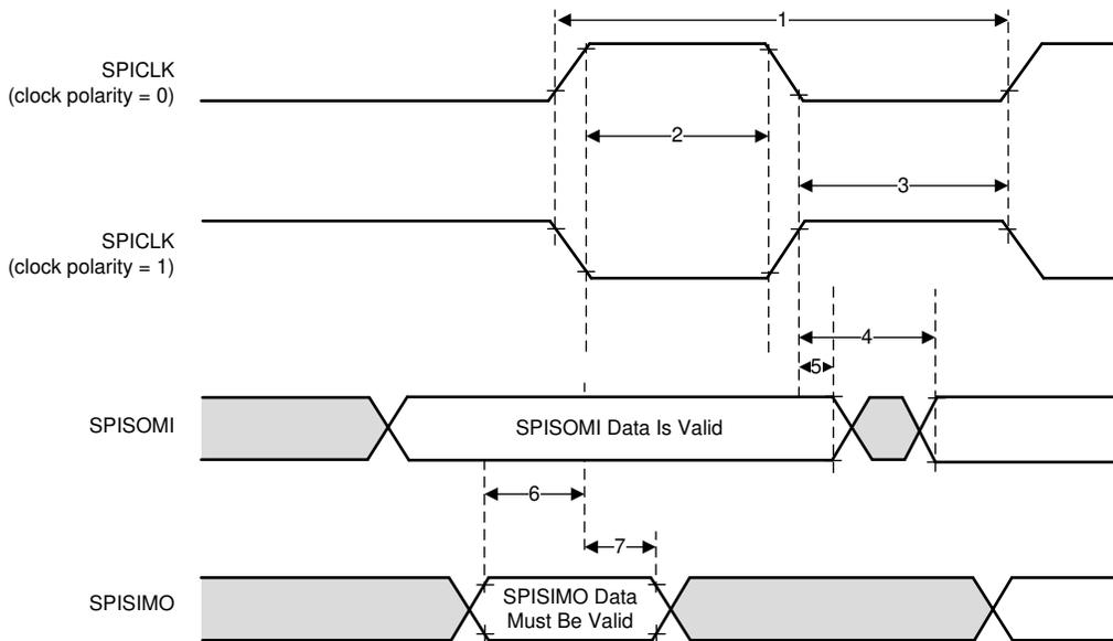
**Figure 7-8. SPI Slave Mode External Timing (CLOCK PHASE = 1)**
