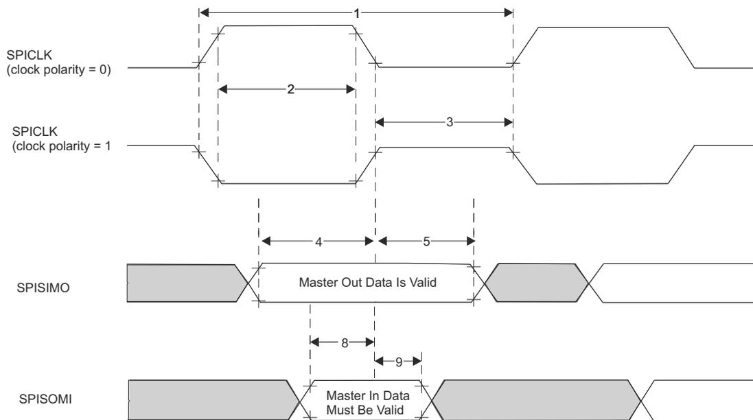
Figure 7-3. SPI Master Mode External Timing (CLOCK PHASE = 0)
