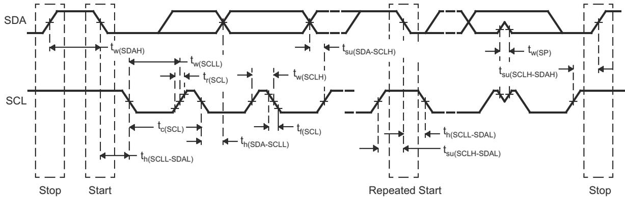
**Figure 7-12. I2C Timing Diagram**
