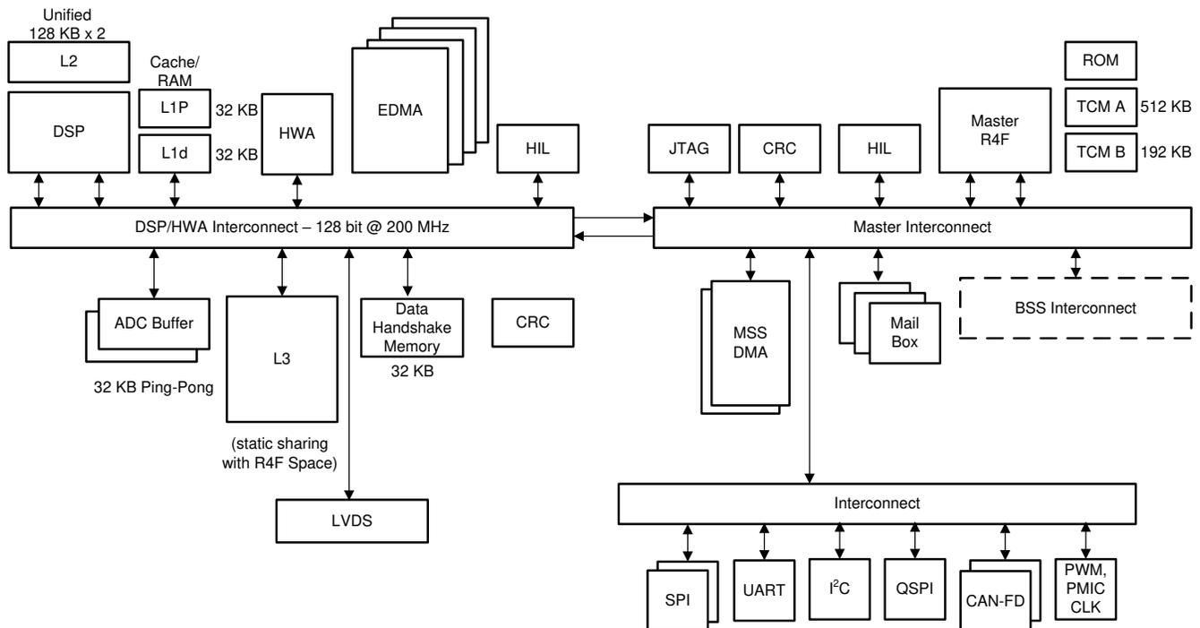
**Figure 8-5. Processor Subsystem**
