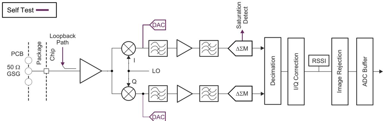
**Figure 8-4. Receive Subsystem (Per Channel)**
