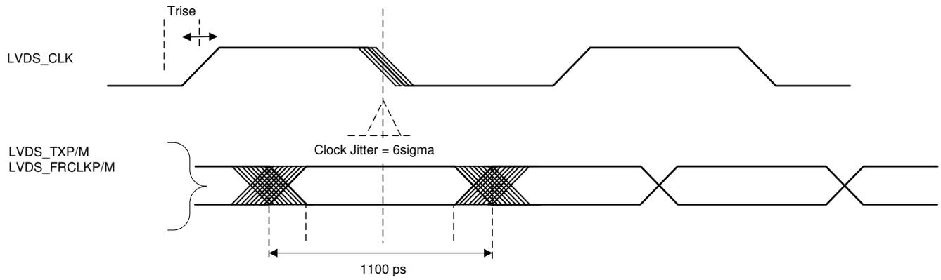
**Figure 7-11. Timing Parameters**
