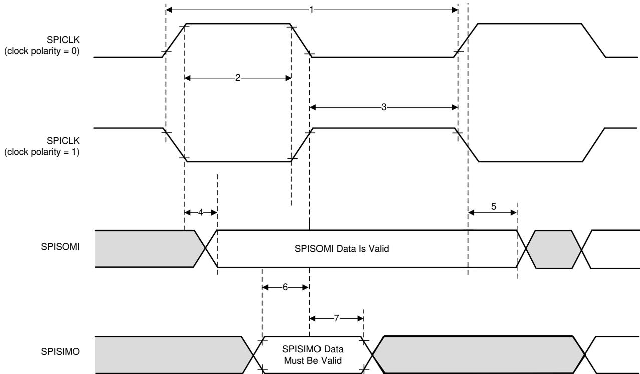
**Figure 7-7. SPI Slave Mode External Timing (CLOCK PHASE = 0)**
