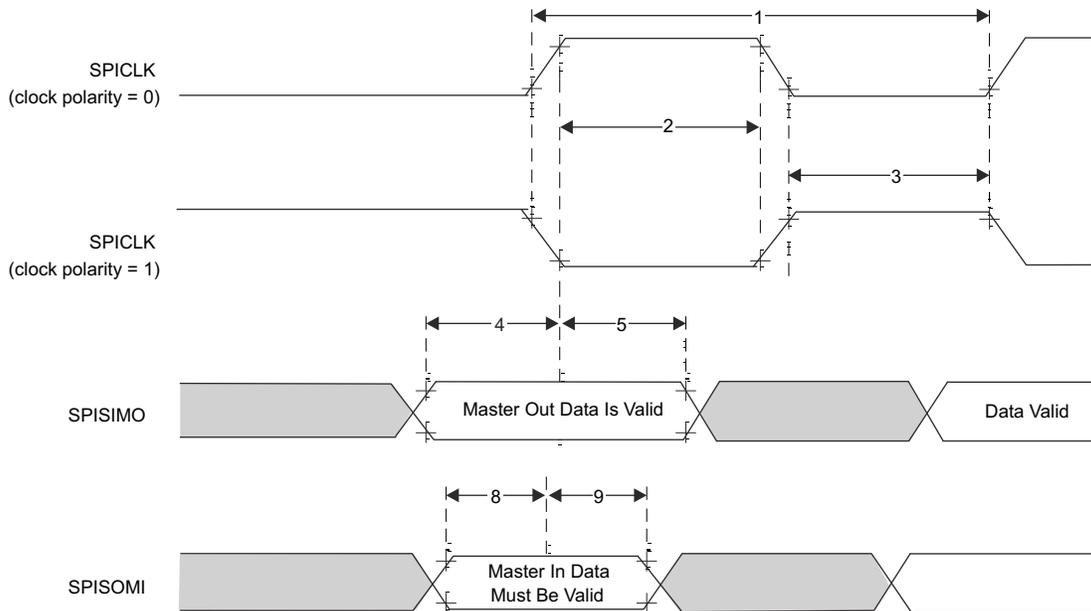
**Figure 7-5. SPI Master Mode External Timing (CLOCK PHASE = 1)**
