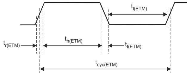
Figure 7-15. ETMTRACECLKOUT Timing
