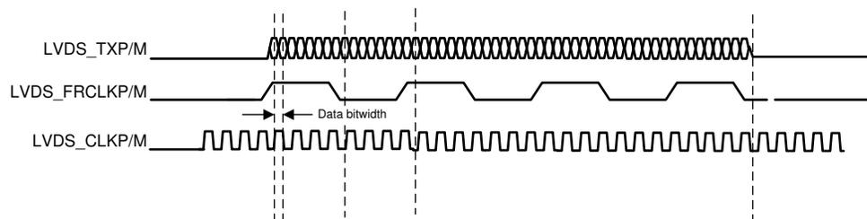
**Figure 7-10. LVDS Interface Lane Configuration And Relative Timings**
