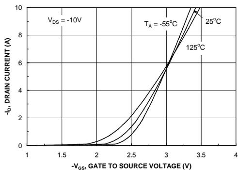
Figure 5. Transfer Characteristics.
