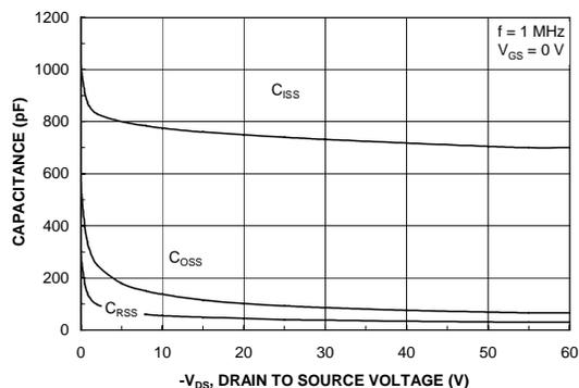
Figure 8. Capacitance Characteristics.
