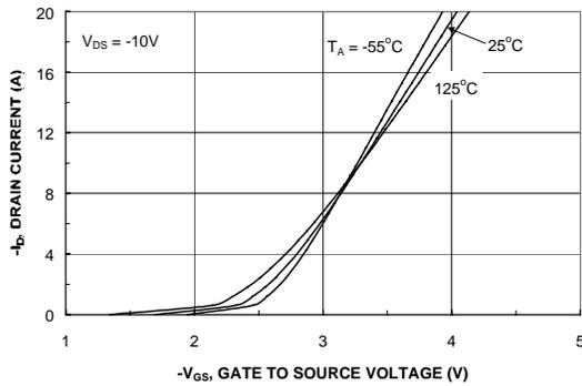
Figure 5. Transfer Characteristics.
