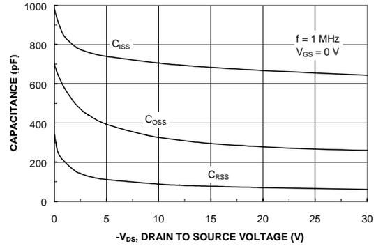
Figure 8. Capacitance Characteristics.
