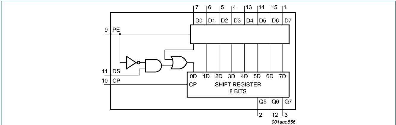
Fig. 1. Functional diagram
