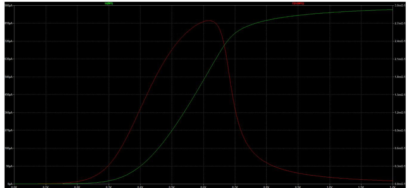
gm and Drain current depending on  $V_{GS}$
