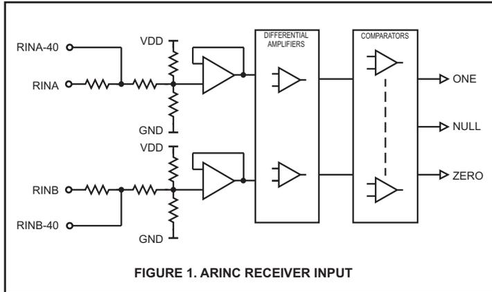
The HI-3588 guarantees recognition of these levels with a common mode voltage with respect to GND less than  $\pm 30V$  for the worst case condition (3.15V supply and 13V signal level). Design tolerances guarantee detection of the above levels, so the actual acceptance ranges are slightly larger. If the ARINC signal (including nulls) is outside the differential voltage ranges, the HI-3588 receiver rejects the data.
