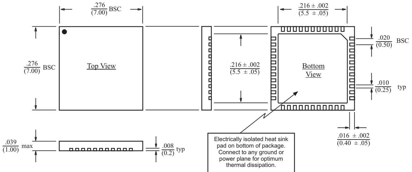
BSC = "Basic Spacing between Centers" is theoretical true position dimension and has no tolerance. (JEDEC Standard 95)
