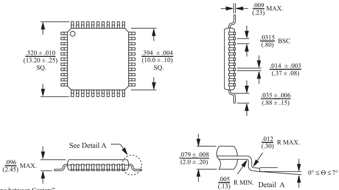
BSC = "Basic Spacing between Centers" is theoretical true position dimension and has no tolerance. (JEDEC Standard 95)
