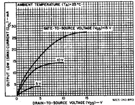
Fig. 1—Typical n-channel output low (sink) current characteristics.
