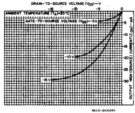
Fig. 3—Typical p-channel output high (source) current characteristics.
