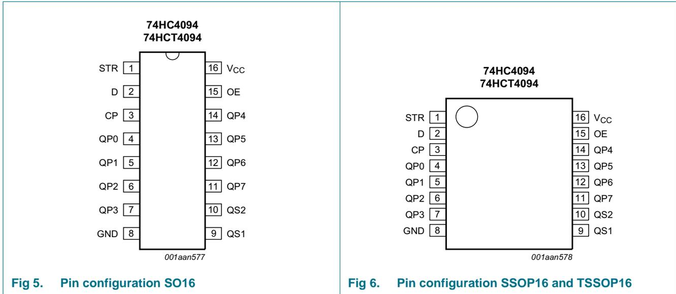
Fig 5. Pin configuration SO16
