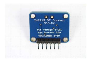
Wires can be soldered directly to the holes on the edge of the board. But for breadboard use, you will want to solder on the included 6-pin header.
