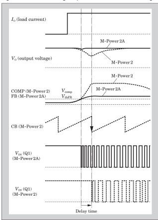
Fig.4 Schematic drawing of operation at sudden load change
