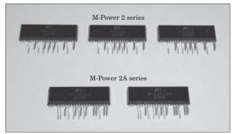
and M-Power 2A series devices. These devices use the same package construction. The M-Power 2A series features improved control IC functionality, and its pin layout differs from that of the M-Power 2 series.
