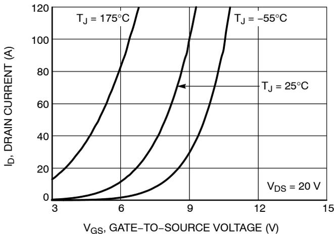
Figure 5. Transfer Characteristics
