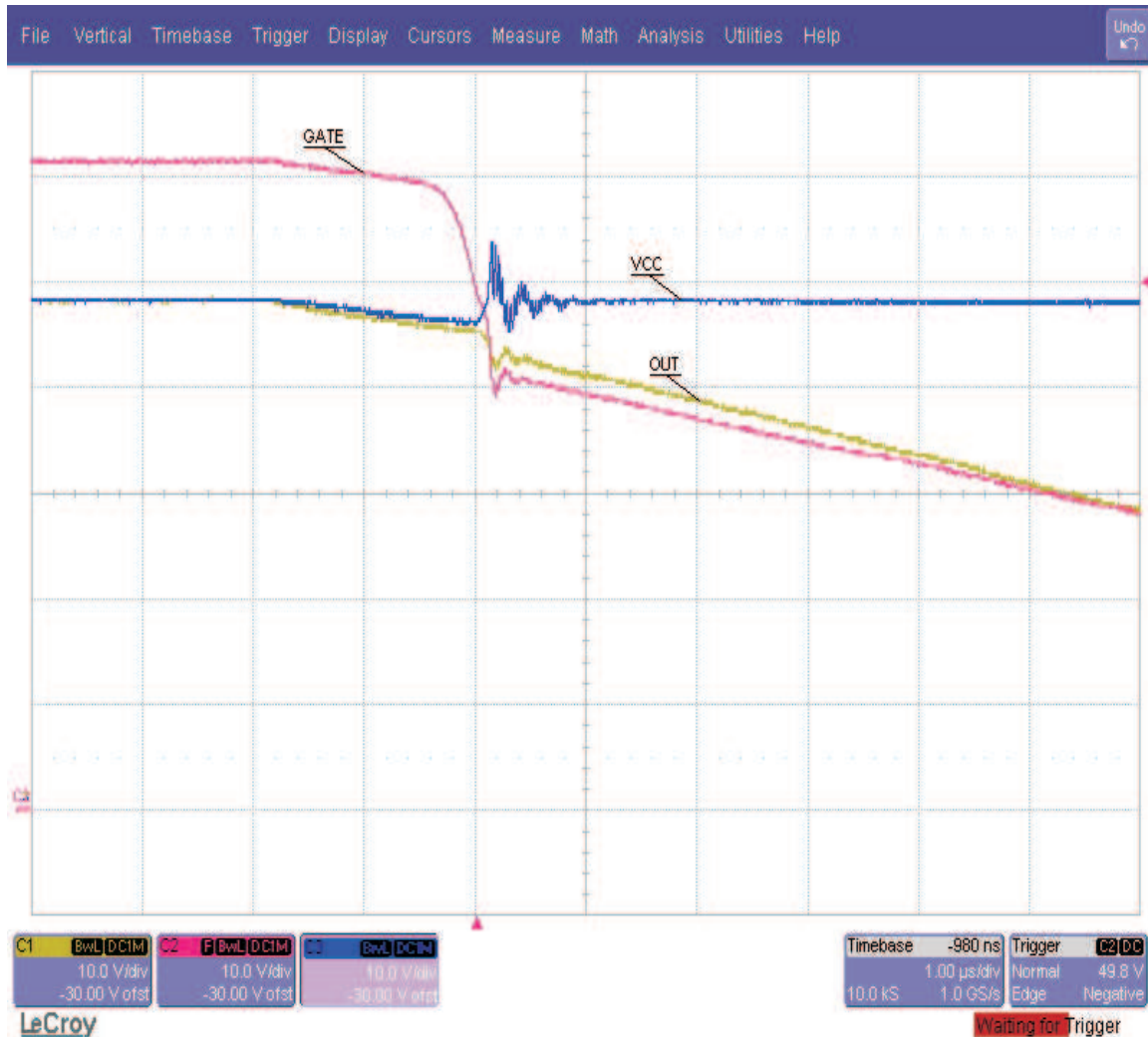
Figure 15. Current Limit Onset
