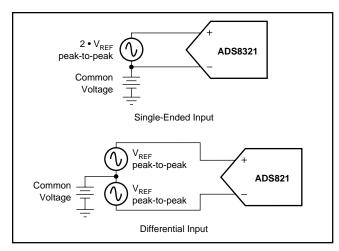
FIGURE 1. Methods of Driving the ADS8321—Single-Ended or Differential.
