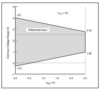
FIGURE 3. Differential Input—Common Voltage Range vs  $V_{\text{REF}}$
