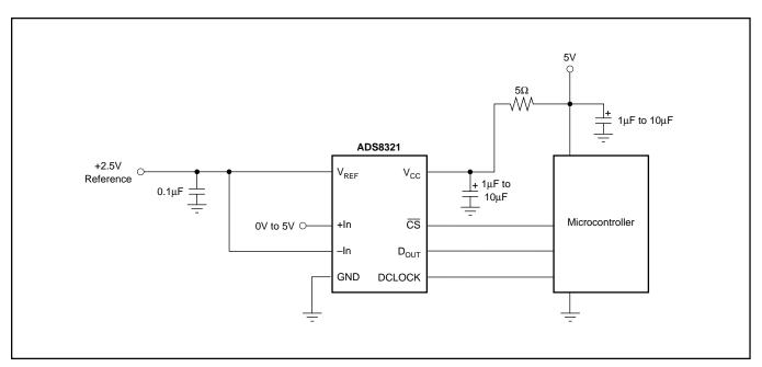
FIGURE 11. Basic Data Acquisition System.
