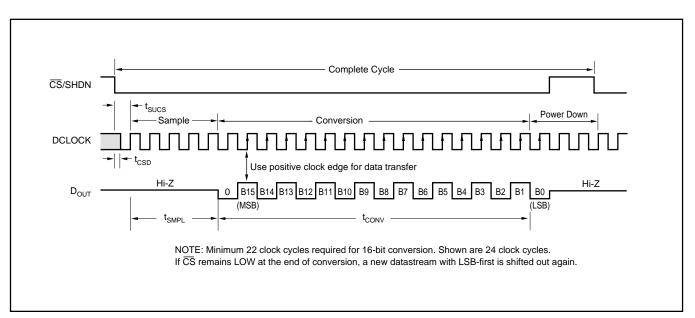
FIGURE 6. ADS8321 Basic Timing Diagrams.
