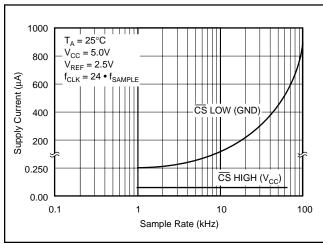
FIGURE 10. Shutdown Current with  $\overline{\text{CS}}$  HIGH is 50nA Typically, Regardless of the Clock. Shutdown Current with  $\overline{\text{CS}}$  LOW Varies with Sample Rate.
