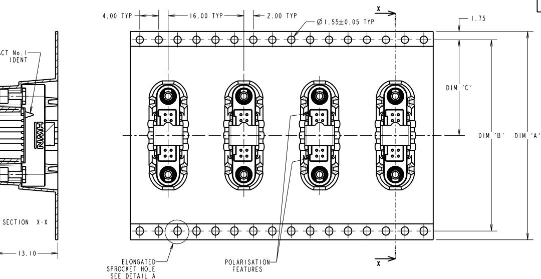
TAPE STRIP DETAILS ONLY. SEE SHEET 3 FOR CONNECTOR AND PCB LAYOUT DETAILS.
