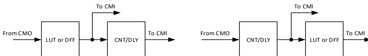
Figure 32. Possible Connections inside Multi-Function Macrocell
