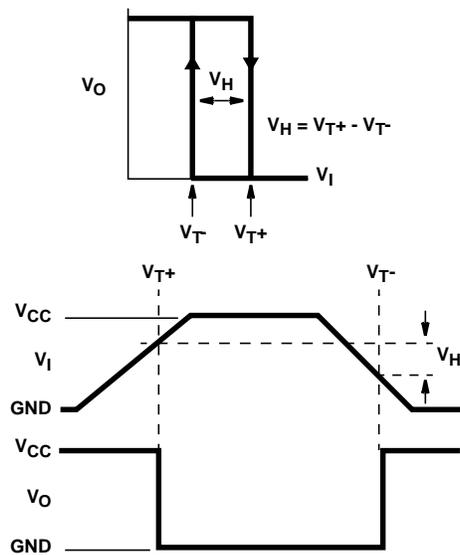
FIGURE 3. HYSTERESIS DEFINITION, CHARACTERISTIC, AND TEST SETUP
