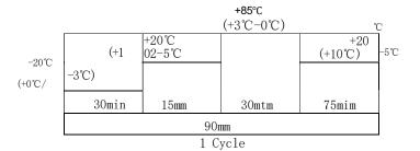
The product was placed in a test chamber at  $-20^{\circ}$ C and another at  $+70^{\circ}$ C for 30 minutes each. min,For one temperaturecycle.
