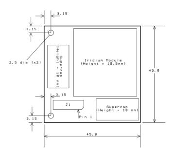
\*Note that the diagram and dimensions do not include the SMA connector
