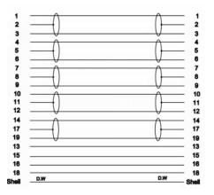
CABLE SPEC;(0.254mmCCS\*1Pair+0.254mmCCS D.W.+AL+MY)\*5+0.254mmCCS\*4C+0.254mmCCS D.W. +AL+16\*6\*0.12mmAL-Mg Braiding)\*1C O.D:6.0mm BLACK PVC JACKET
