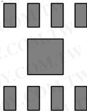
Figure 3 (a). Minimum Footprint,  $\theta_{JA} = 75^{\circ}\text{C}/\text{W}$
