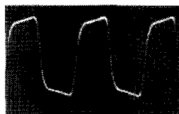
Fig. 17(c) - CA3070 terminal No. 8, oscillator waveform 1.6 V p-p 3.58 MHz.
