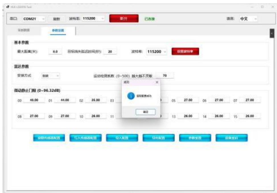
Figure 4 — Millimeter-Wave Sensor Parameter Reading Interface
