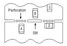
(3) Mounting components near screw holes
