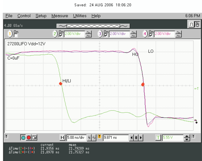
Figure 32. V_{LO} and V_{HO} Falling Edge Delay Matching
