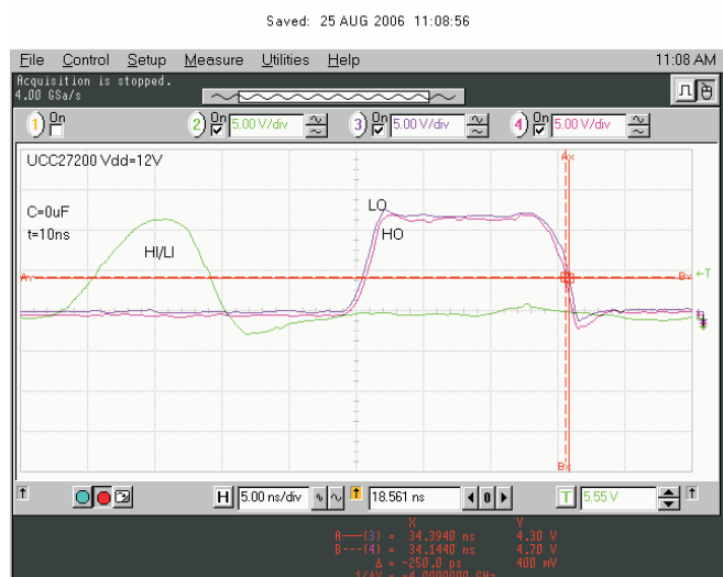
Figure 34. 10-ns Input Pulse Delay Matching
