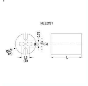
PVC round LED spacer for use with T-1(3mm) LED; available in lengths of 4.8-30.0mm
