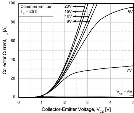
**Figure 2. Typical Saturation Voltage Characteristics**
