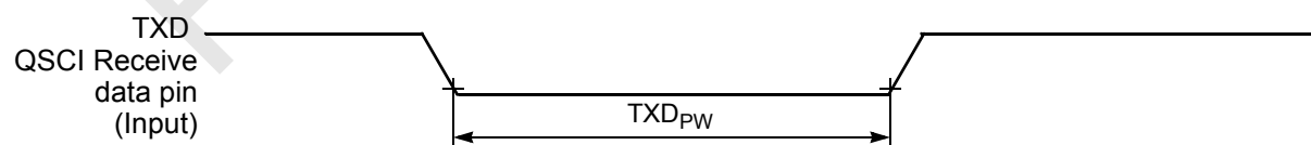
Figure 10-13 TXD Pulse Width
