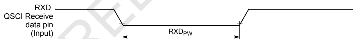
Figure 10-12 RXD Pulse Width
