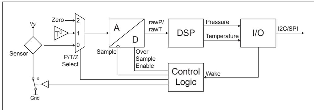
The ADC performs conversions on the raw sensor signal (P), the temperature reference (T) and a zero reference (Z) during an ADC zero cycle. It also has an oversampling mode for a noise reduced output. A conversion cycle that is measuring pressure is called a Normal cycle. A cycle where either a temperature measurement or zeroing is being performed is called a Special cycle.
